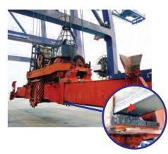
The extension frames supported by sliders such that they may contact with each other through sliding motion. Due to the intensive surface contact, the sliders become worn and prevent them from functioning properly. The use of specialized lubricant can significantly help to reduce wears and corrosion.
