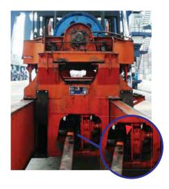
The chain lubricants help to protect the spreader chain from wears and providing resistance to corrosion especially when exposing to extreme weather condition and seawater.
