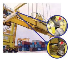
The guide arm can be swung from upper, turned-over open position into position for engagement with a corner of the container. Corrosion may cause the friction and obstruction to the movement of the guide arm. We offer TACBECON SG 1000S which has the ability to prevent the inception of corrosion when exposing to weather and saltwater environment.
