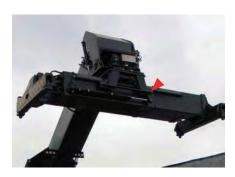
When carrying heavy load, the side shift of the top pick spreader requires lubricant to reduce wears caused by friction in sliding contact. Formulated extreme pressure additive, TACBECON SG 1000S grease leaves a stronger film strength to protect the mechanisms from high-loading pressure.
