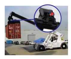
TACBECON SG 1000S is recommended for use in exposed gears. This lubricant is ideal for gears when operating under heavy loading pressure and outdoor conditions as it provides a tacky lubricant film that adheres to gear surfaces so as to protect against corrosion, rust, wears and shock load.
