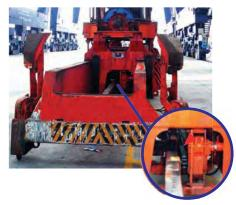
The chain in the spreader is driven by a drive to extend or contract the lateral extension frames that allow a variety of containers with different lengths to be suspended. Due to intensive surface contact, the chain components wear off easily.
