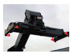
TACBECON SG 1000S can be applied on the top pick spreader twistlock mechanism because it leaves a stronger film strength on the metal surface to protect the mechanisms from high-loading pressure.
