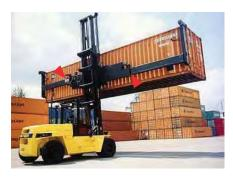
TACBECON SG 1000S, a heavy duty grease, can be applied to reduce the sliding friction in the telescopic side spreader as well as to protect the metal part from corrosion especially operating in the seaport environment.
