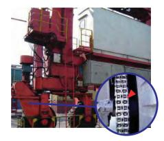
The power chain in the wheel assembly drive the RTG crane to move from one location to another. It is important to apply lubricant to protect the power chains from seizure and damages.
