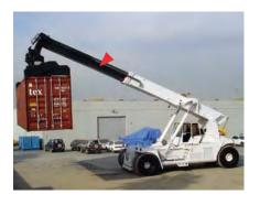
TACBECON SOG 3000A is an excellent choice for telescopic boom application as it contains superfine graphite that not only helps in cushioning shock loads but it helps in smoothening the irregularities of pad-to-boom surfaces for smoother operations. In addition, this lubricant has longer service life which keeps the wear pad of the boom lubricate for a long period of time before relubrication.
