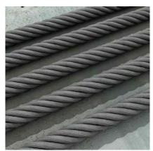
Many users normally believe that by coating heavily onto the surface will give a better protection to the wire rope. However, most of the wire rope fail from inside, it is important to make sure that the center core receives sufficient lubricant.
